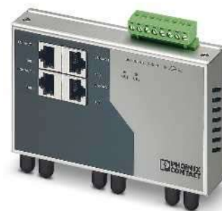
4 RJ45 ports and 3 FO ports
