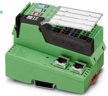
RJ45 connection, 8 digital inputs and 4 digital outputs
