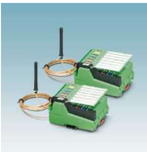
Bluetooth wireless modules (2.4 GHz) Wireless multiplexer with antennas Page 466
