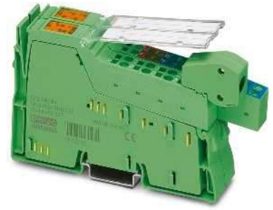
Input for incremental encoder with square-wave signal (symmetrical or asymmetrical)
