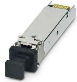
Fiberglass, for Gigabit transmission ranges up to 2 km
