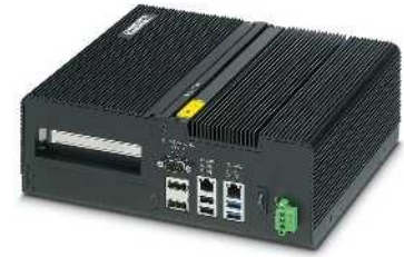
Box PC with Intel® Core™ i3-4010U technology and PCI/e slot
