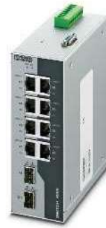
8 RJ45 ports and 2 SFP ports
