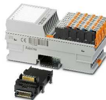
2 counter inputs, 2 incremental encoder interfaces
