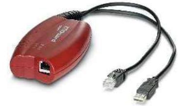
Router with firewall for mobile use
