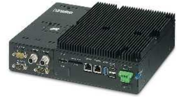
Box PC with Intel® Atom™ E3845 technology
