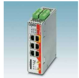
Remote maintenance – mGUARD security router
