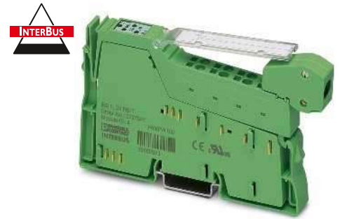
Remote bus branch via copper cable
