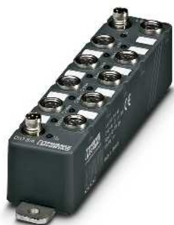
4 digital inputs and 4 digital inputs or outputs
