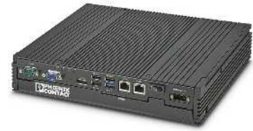
Box PC with Intel® Celeron® N2930 technology and PCI slots
