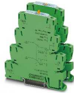
Module with manual switch without relay
