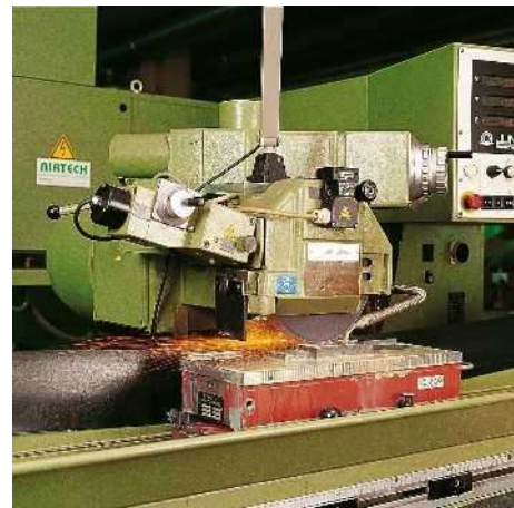
Protection against blocking and broken tools, warning thresholds for tool and bearing wear.
